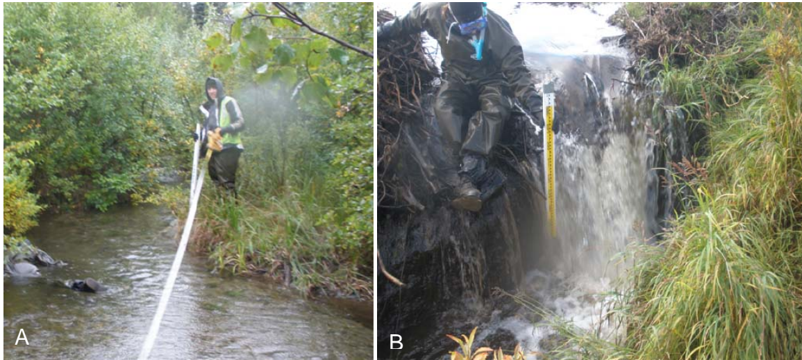
PHOTO 40.1-1: Habitat surveys to document the types and quality of aquatic habitats present in the transportation corridor study area were conducted. Habitat unit measurements were collected with a 165-foot (50-meter) Kevlar tape (A) and a stadia rod (B).
