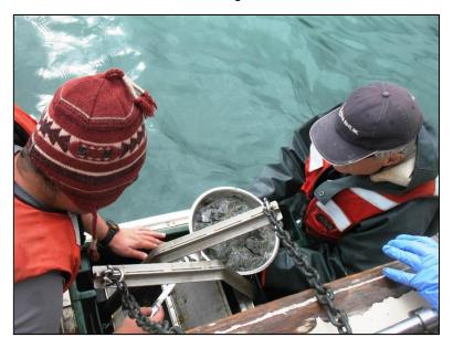
Benthic sediment sample collection with a Van Veen bottom sampler,  $\mbox{\it July}, 2008$
