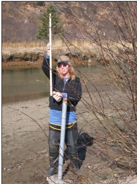
PHOTO 31-2: Checking staff inside crest gage for peak flood data at No-Name Creek near North Head (Y Valley).
