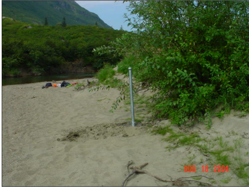
PHOTO 31-1: Example of newly installed crest gage at No-Name Creek near North Head (Y Valley).
