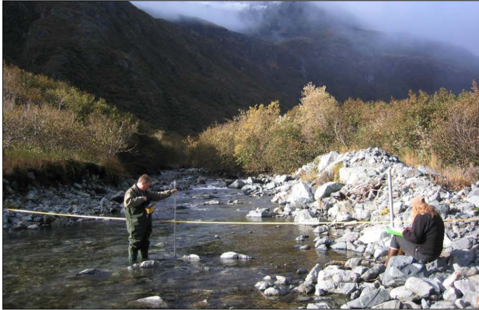
Field crew taking a discharge measurement using the wading method on Williams Creek.
