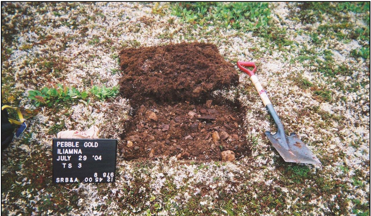
PHOTO 22-23: Test Unit TS-04-03 shows fractured gravel just below the surface mat. July 2004.
