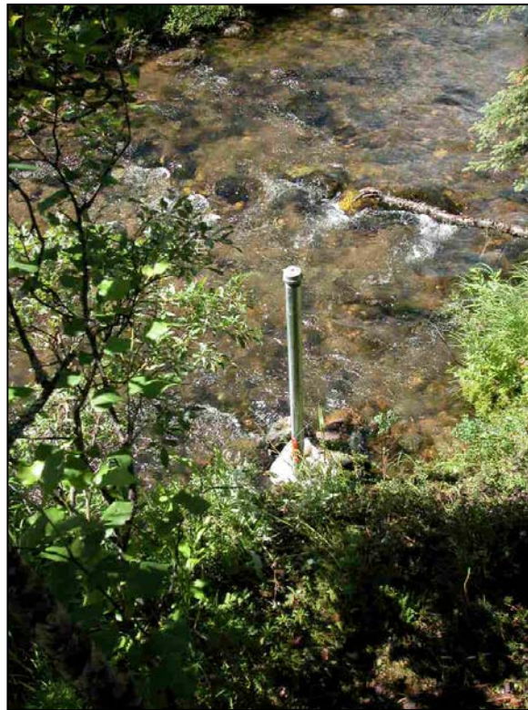
PHOTO 2: GS-14a Unnamed Creek East of Eagle Bay Creek. View looking down on new set of gage during low flow, July 19, 2004.
