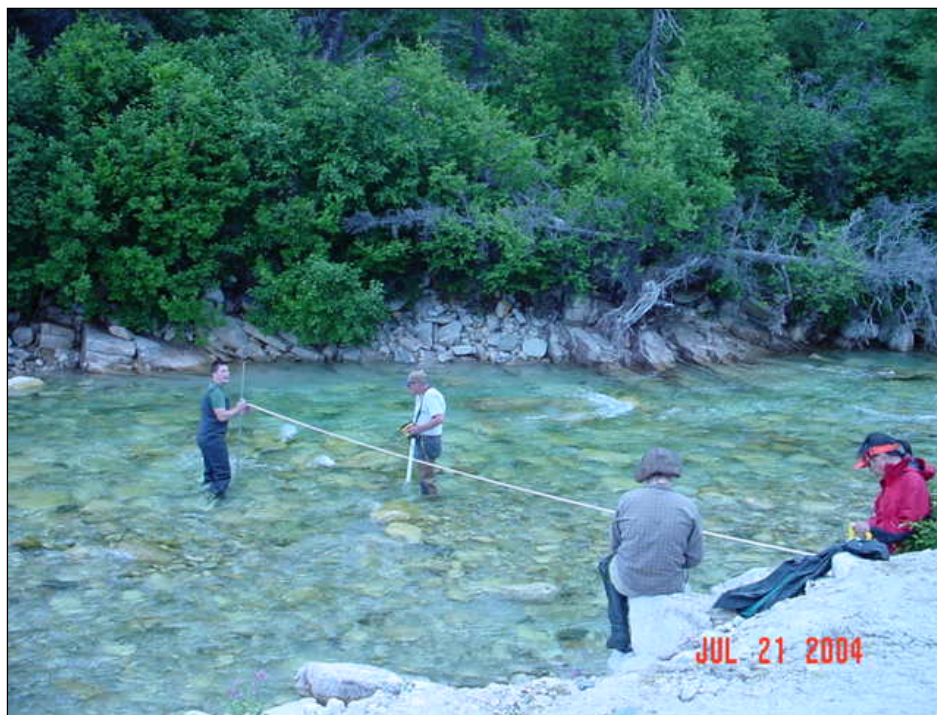
PHOTO 7.3-3: Field crew taking a discharge measurement using the wading method on Knutson Creek (Gaging Station GS-8a).
