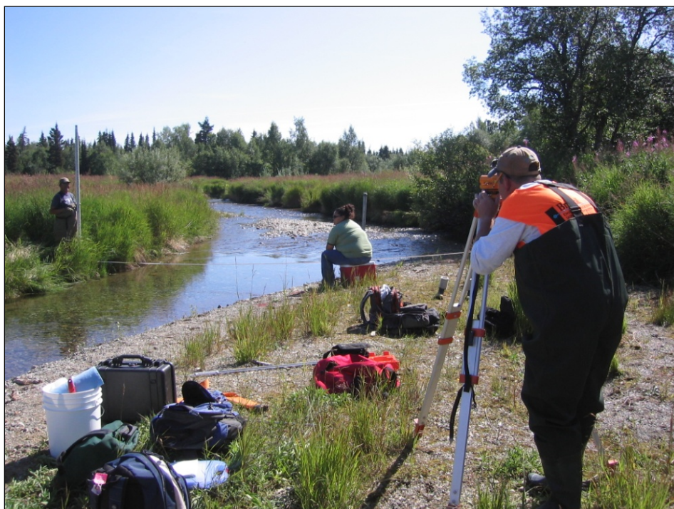
PHOTO 7.3-2: Example of survey for stream cross section.
