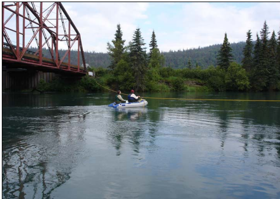
PHOTO 2: GS-3a Iliamna River. Data taken from small boat using a tag line, July 13, 2005.
