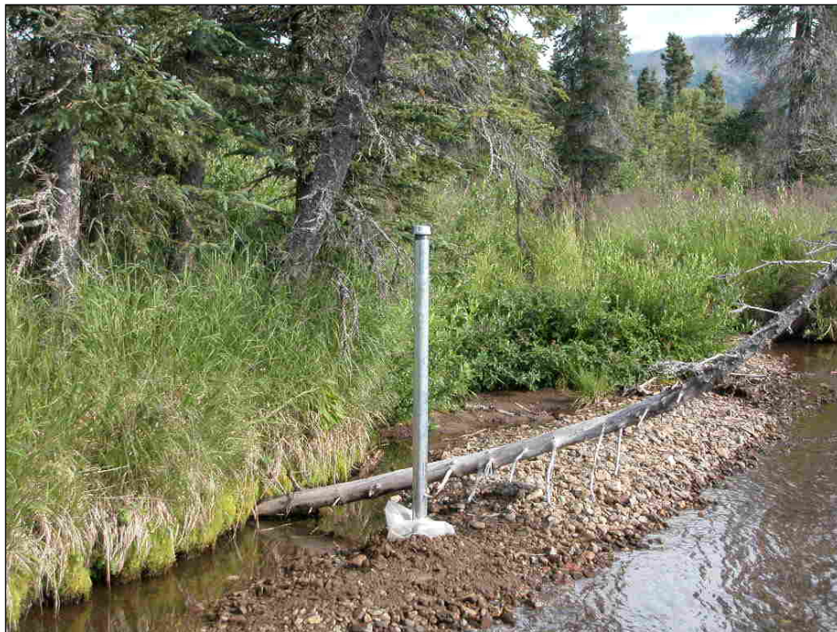
PHOTO 7.3-1: Example of newly installed crest gage.
