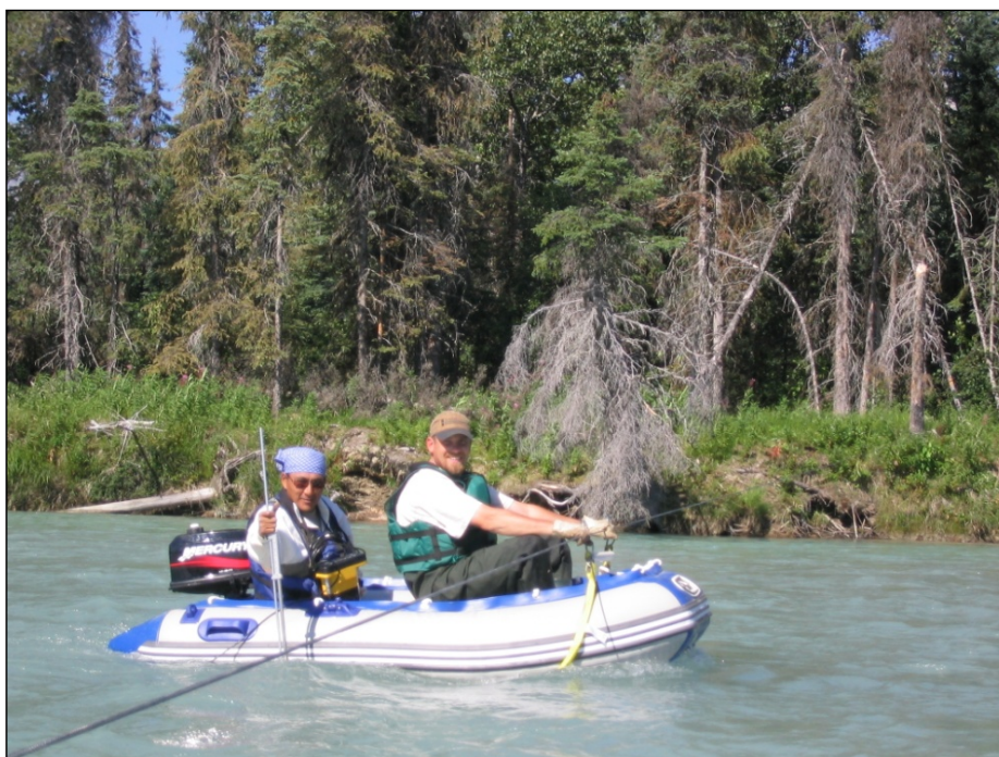
PHOTO 7.3-4: Field crew taking a discharge measurement using a small boat on the Pile River (Gaging Station GS-4a).
