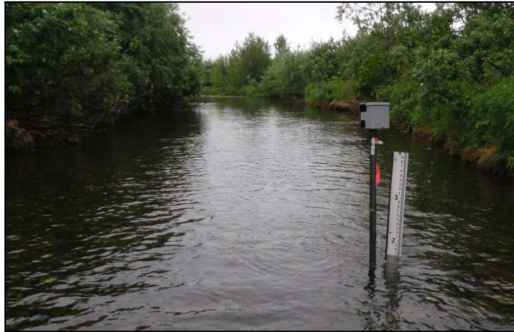
Typical surface hydrology gage installation (SK119A).
