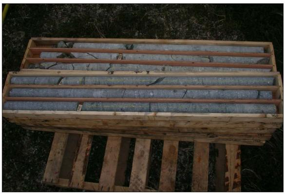
Typical bedrock cores from exploration/geotechnical drilling.
