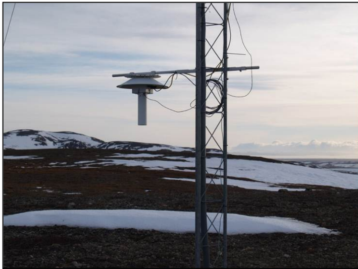
Temperature Sensor at 2 Meters above Grade in the Mine Study Area, February 2007
