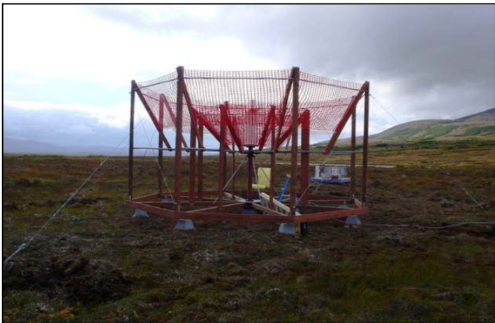
Precipitation Gauge with Wyoming Wind Screen in the Mine Study Area, September 2007
